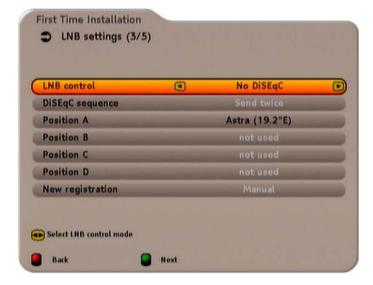
Press the 🔊 buttons to switch to the "Position A". Press the OK button to open the sub-menu. You can select a satellite and make the related settings here. Press the (green) button. If you change the default setting (in this example "ASTRA 19.2°E"), a prompt "Save LNB settings?" will be displayed. Select "Yes" or "No" using the (N) buttons and accept your selection using the (N) button.
